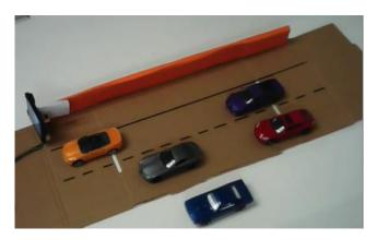
You can use waste corrugated paper to draw a complete lane, and then fix HuskyLens above the emergency lane to ensure that HuskyLens can detect vehicles in it.
