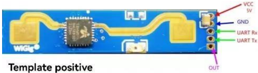
Figure 1 Module pin definition diagram
